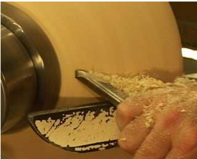
Fairing the curve on the outside of a dry bowl
