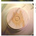
I still have the original center mark from the tailstock to center the bowl by when I reverse to turn the foot.
