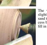
The waste parted off. I cut through slightly away from the bowl bottom and sand the nub off. You can sand away excess but it is harder to add something to fill in a dip if you cut too deep.
