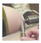
You can see from this view that the top flute of the gouge just clears the surface. This is a scraping cut and will dull the gouge quickly so be prepared to sharpen often for best results.
