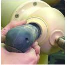
Power sanding the lower area of the bowl to blend in with the top. Stay away from the detailed foot. If you round over an edge you wanted to be sharp go back and cut the edge again.
