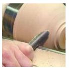
Shear scraping cut. The gouge angled about 45 degrees to the wood surface and the top flute nearly touching the wood. The shear scrape is a light finish cut used to remove ridges or very slightly torn grain. The gouge moves along the wood surface refining the shape and removing any high spots. The gouge can move back and forth over the wood surface. Stop the lathe and check the wood
