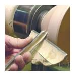
True the wood surface and shape the bowl profile now. If the bowl runs perfectly true after reversing in the chuck you only need to turn enough to make sure you have the finished shape and surface you want. The bowl rarely runs perfect for me when I reverse so I save the finish cuts until the bowl tenon is in the chuck.
