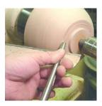
Cutting in toward the tenon to form a square or slightly undercut shoulder against which the chuck jaws can seat.
