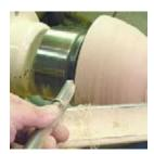
Be careful with sharp edges on spinning wood. Most of my cuts and scrapes have come from contact with a shape edge on the rotating wood. Relieve the edge with the gouge.
