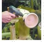
Slow the lathe speed and power sand the bowl. If you have some areas that need special attention, sand them with the lathe stopped and then turn the lathe back on and continue power sanding the whole surface. Do not push hard on the wood or keep sanding with a clogged piece of paper. The sandpaper needs to cut the surface not burnish it. You do not want to generate a lot of heat the wood
