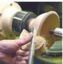
Shear scraping to remove any torn grain. I leave the tailstock in for support until time to start hollowing. With cross grain turning the wood could split parallel to the face of the chuck if a big catch occurs or when turning large heavy bowls without the tailstock for support.
