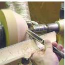
Taking a lighter finishing cut with the bowl gouge angled higher up on the blank with the bevel near the rubbing. The shaving comes off the lower tip of the gouge.
