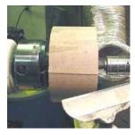
I call this turning a simple bowl because I am not using any special tools just bowl gouges and spindle gouges. The shape is a simple one also. I know that when you first start turning bowls trying to get the surface cut cleanly on the end grain areas can present a problem. Reversing the bowl to finish the bottom can also present a challenge.
