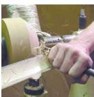
Using an overhand push grip for a little more strength behind the cut. Put pressure down on the tool rest and steady pressure and control in the line of cut.
