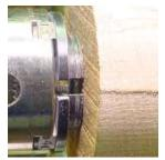
The blank compressed between the chuck jaws and the tailstock center. Stuart Batty demonstrated this technique for our turning clubs. This technique works well for blanks cut from even thickness slabs in bowl and platter turning.
