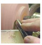
Cutting the straight tenon to fit in the chuck jaws. This would also work for tuning a tenon to glue in the recess of a waste block on a faceplate.
