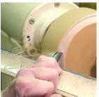
I start rough shaping the bowl shape from the tailstock end. I oriented the blank with the wood I want to be at the bottom of the bowl on the tailstock end on purpose. I have more room to turn down to a small diameter on the tailstock side than the headstock side. This makes turning the tenon for the chuck or faceplate easier.
