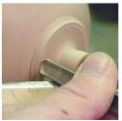
Using the spindle gouge to define the foot edge thickness.
