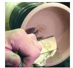
The center of the bowl spins at slower feet per minute speed than the outer edge. Slow the advance of the gouge to compensate for the change.
