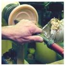
Continue hollowing the bowl until you get close to the wall thickness you want in the top area of the bowl. Leave the bottom section of the bowl thick at this stage.
