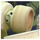
I am going to reverse the bowl on to a jam chuck that fits in the interior of the bowl curve. Make the jam chuck from a wood that is softer than the turned bowl and round the edges of the jam chuck to help prevent marring the finished piece. This also works with natural edge bowl because it does not rely on the bowl rim for support.
