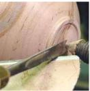
Using a shallow carving gouge to part through the last of the waste area of wood. This can be done while rotating the lathe by hand. David Ellsworth shows this technique on his turning videos, the first place I saw this technique demonstrated.
