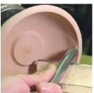
I reverse the lathe rotation to cut the top of the bowl wall. This brings the tool handle back over next to my body for more comfortable turning and better tool control.
