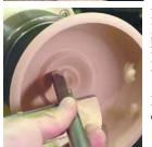
Deeper in the bowl now I reverse the lathe rotation back to normal so the tool handle comes back to the front of the lathe near my body for more comfort while turning.
