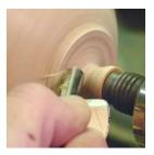
Remove the wood in the center to below the foot edge level. You can shape the inside of the bottom to be convex and mirror the interior of the bowl or concave if you have allowed enough wood thickness.
