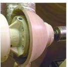
The bowl compressed on the jam chuck and centered on the tailstock end.
