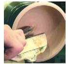
Take your time and remove the center. The curve on the inside should be continuous from side to side without bumps and flat spots. Use your fingers to feel for flat areas and if found take light cuts to remove them.
