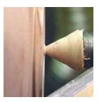
Reduce the waste at the bottom in preparation for parting off.
