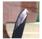
The long bevel on this gouge interferes in the cut by rubbing on the bowl wall so I ground part of the lower bevel away until I could get the edge in the cutting position I wanted with no bevel interference.
