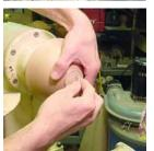
The jam chuck holds the bowl well enough for me to turn the lathe on slow and support it by hand for a little final sanding.
