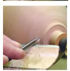
I am going to turn a small detailed area for the actual foot. I am cutting against the grain with a small spindle gouge to define a transition from bowl side to foot.
