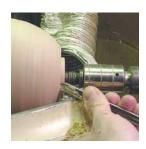
My ½" bowl gouge is sharpened to the profile of a spindle gouge with a total angle of bevel and flute less than 90 degrees. I use this gouge for turning the tenon and shoulder because it can cut into the tight transition area.
