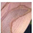
The finish cut surface on this section of the bowl. Check to make sure there are no torn grain areas and then continue to hollow further toward the center. Do not allow the trailing bevel of the gouge to leave burnished ring marks in the wood either. Try for a uniform clean-cut look to the wood surface. Sanding and applying finish will go much easier if you do.
