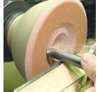
The bevel of the gouge points in the direction if the cut. The flute of the gouge is rolled back slightly up to allow the cut to come off the lower edge near the center of the gouge.
