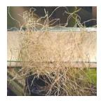
The shavings produced from the finishing cut. The finish cut is a shearing type cut and can produce fine tight curled shavings.
