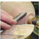
Shape the bottom section of the bowl to blend in with the rest of the bowl profile.
