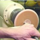
Set the tool rest so the center of the gouge, with the handle horizontal, hits the bowl center or slightly below. If the gouges tip hits, above center, the handle will have to be raised to cut the center and that gets uncomfortable if your lathe spindle height is already high.
