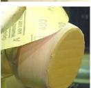
I use a piece of self-stick sand paper with the grit side to the bowl surface. The fine grit will not damage the surface unless you get a big catch and spin the bowl on the jam chuck.
