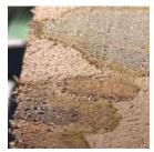
The torn endgrain area of the blank left after using a heavy roughing cut with the bowl gouge. This area needs to be gone over with a freshly sharpened tool and light cuts to get past the depth of the torn grain.
