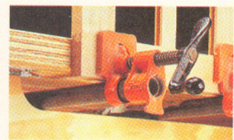
◀ Pipe Clamps. To hold a workpiece against the edge of the bench, slip pipe clamps through the notches at the top of the stretchers.
