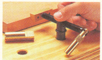
◀ Bench Dogs. Using one (or more) pairs of bench dogs lets you hold work tightly against the top without clamps getting in the way.
