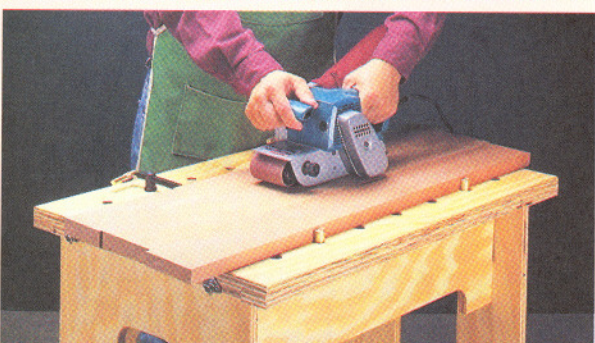
◀ Bench Dogs. Using one (or more) pairs of bench dogs lets you hold work tightly against the top without clamps getting in the way.
