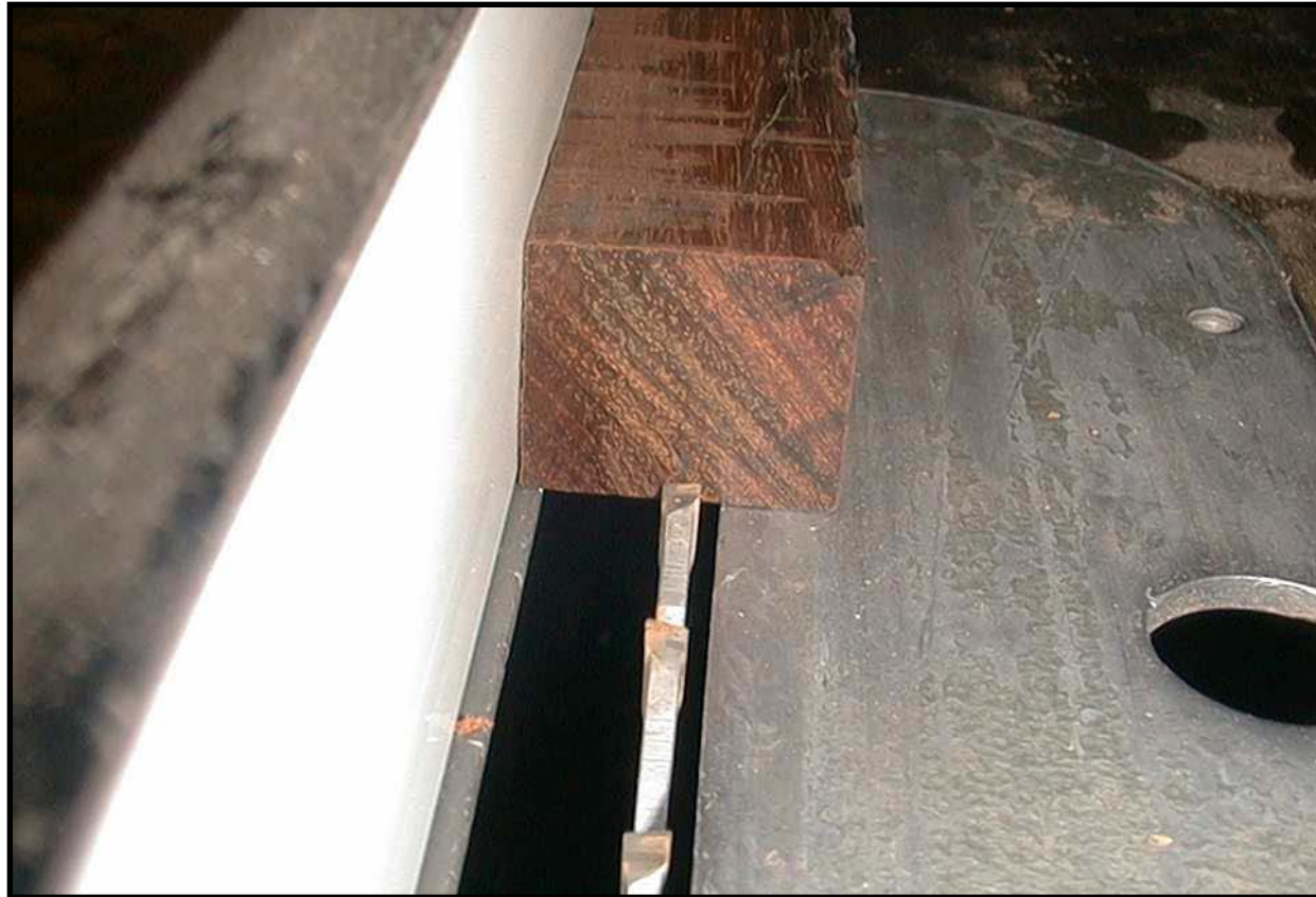
Setting up to cut a groove
