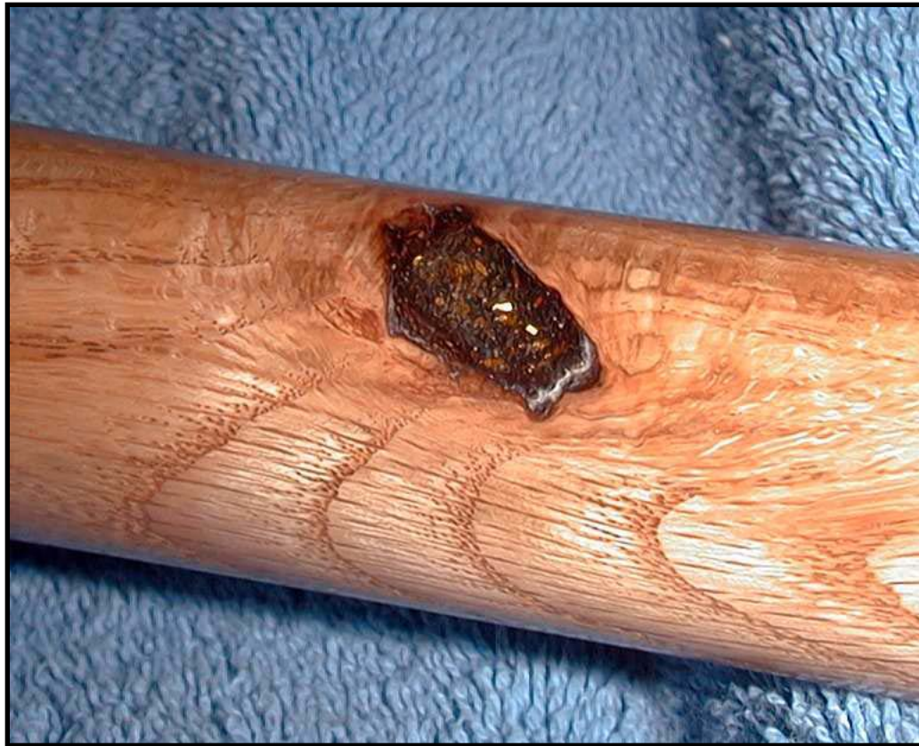
Epoxy fill of knot with metallic flake
