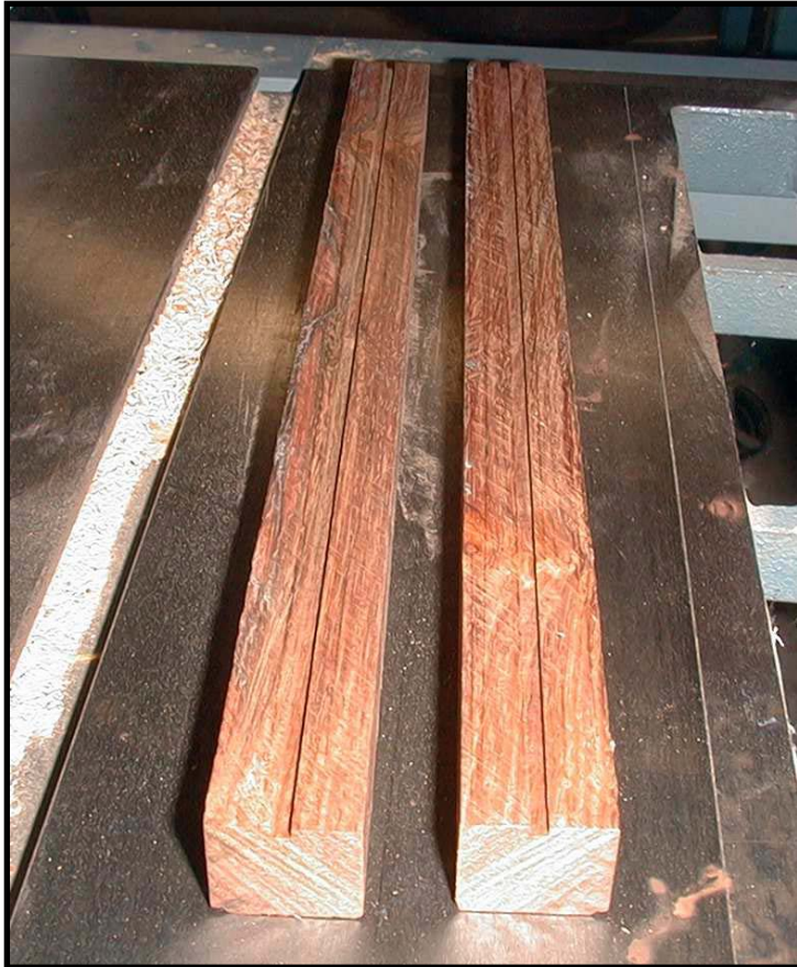
Groove cut in two halves to form core of handle
