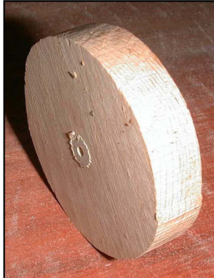
Dowel pushed into end cap
