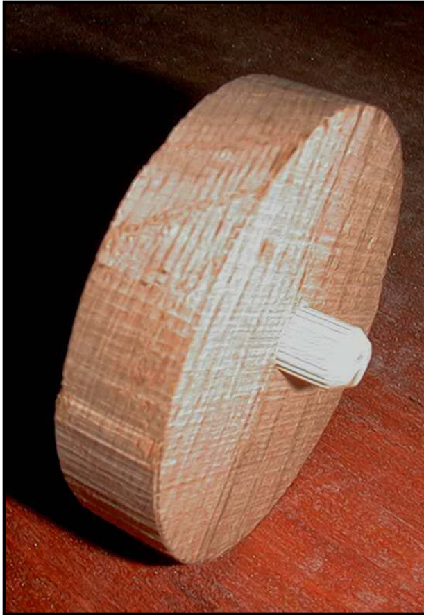
Dowel pushed into end cap
