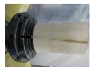
Mount in the pot chuck in the chuck. True up and bring the diameter to 2". Face the end flat.
