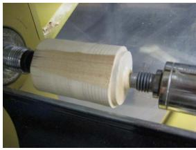
Turn the corners off so that the diameter is 2"-2 1/8". Face the end flat and make the dovetail 1 7/8" diameter by 3 /16" long or make a spigot to fit your chuck.
