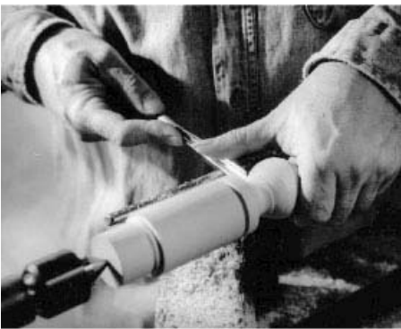
Using the hand to steady vibration
