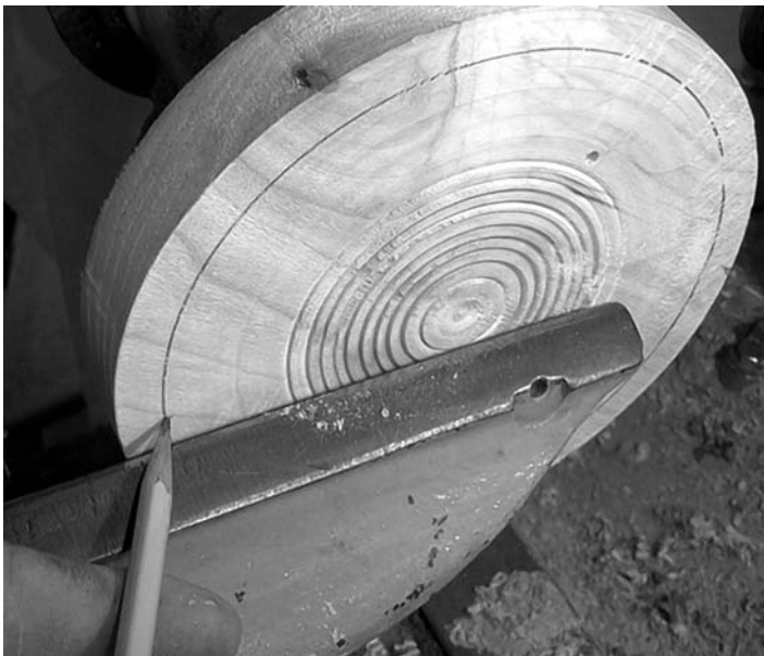
Scribe lines every \frac{1}{2} -in on the mounting disk to aid in aligning the workpiece.
