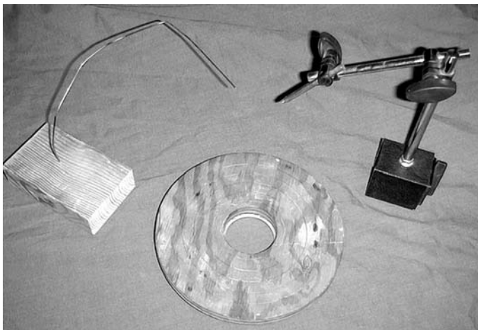
The author's centering method requires a disk for mounting faceplates and a simple pointer, either shop-built, left, or a commercial model, right. Photos by author
