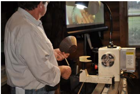
With some simple rotary carving within defined lines along with a black milk paint burnished off, creates the illusion of a fluted bowl.
