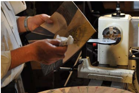
Removing excess paint/burnished paint off
