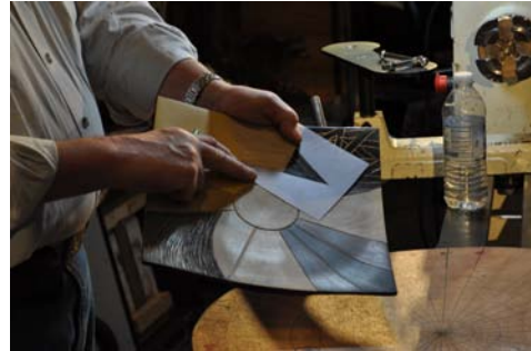
A plastic template is used to mark lines on a painted surface in a geometric manner.
