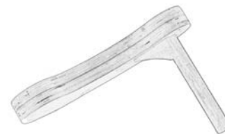
Another plastic template is used as a spatial relationship for the hand of carving. Having registration lines allows the carving to stay consistent.
