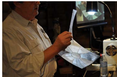
Another plastic template is used as a spatial relationship for the hand of carving. Having registration lines allows the carving to stay consistent.
