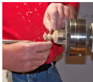
Final sanding on the cap
