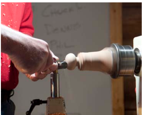
Next the hollowing begins. The piece of wood Gary chose contained a crack which made it very difficult to complete without breaking.
