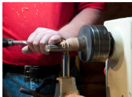
Here Gary is parting off the globe which he did complete without breaking.
