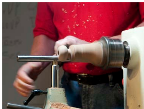
Here Gary is parting off the globe which he did complete without breaking.
