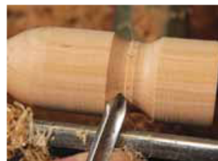
A spindle gouge cleanly cuts coves.
