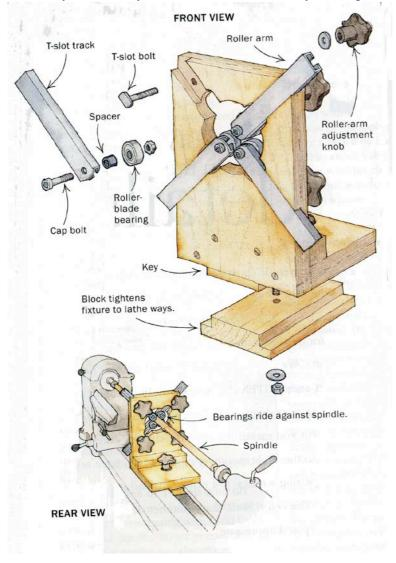
lathe. You will need to tailor the key and the fixture's bed-locking mechanism to your lathe.
